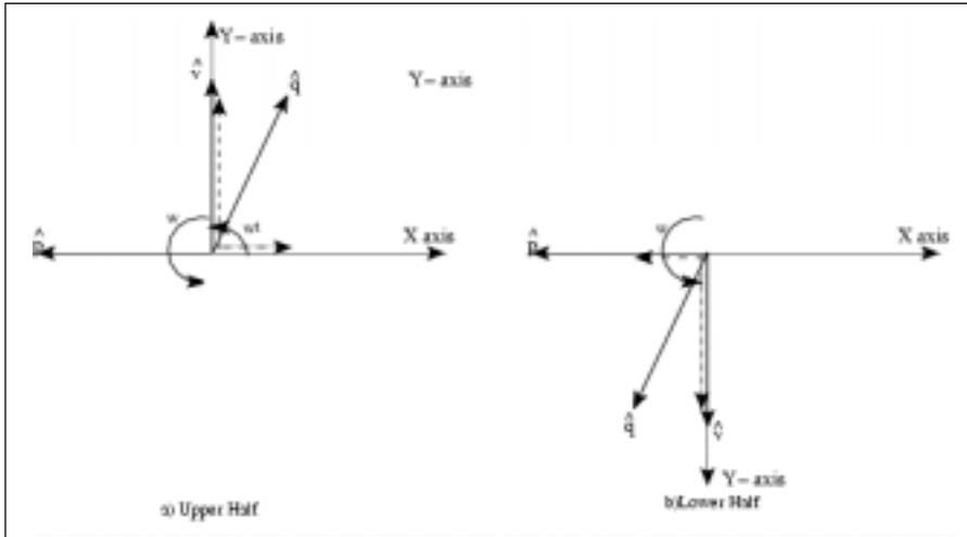
**Figure 5. Phasor diagram for standing acoustic wave in open-open tube.**
