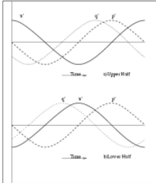
It then only remains to determine the locations within the Rijke tube, where the heat source can drive the acoustic waves.
